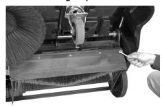
→ Loosen the fastening screws of the sealing strip.
