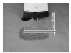
The sweeping track should have an even rectangular shape which is between 30 and 40 mm wide.
