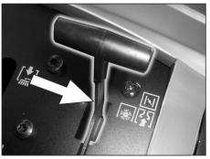
Slide the multifunctional lever into the center position "Operation speed"; if the weather is cold or wet, move it to the "Choke" position.
