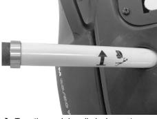
→ Turn the push handle lock counterclockwise: lock is unlocked.
